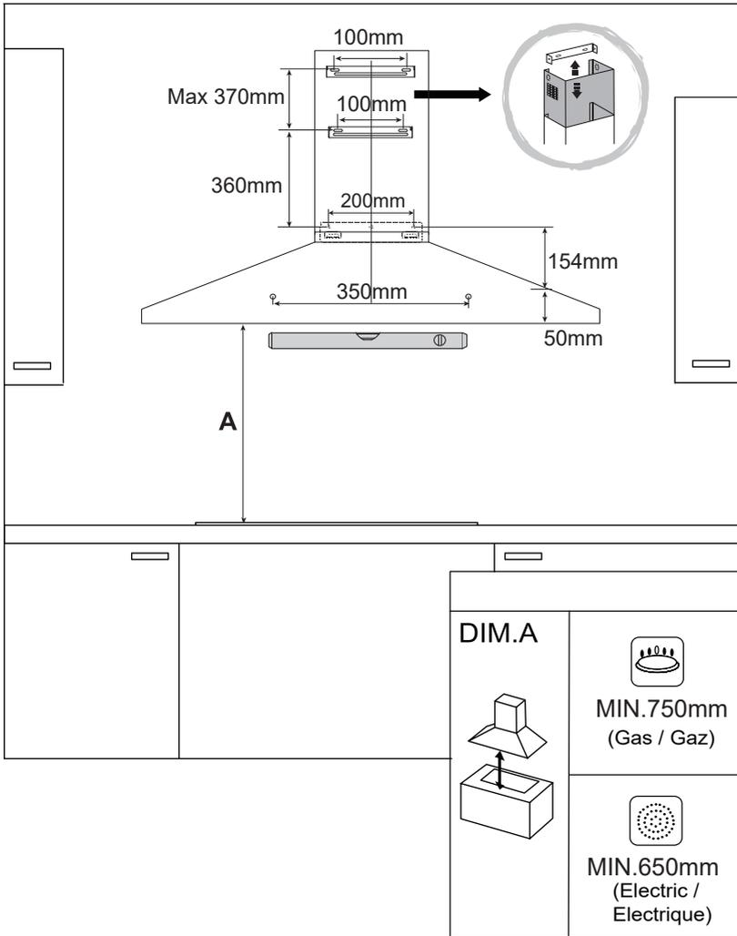
**EN** Mark the wall with the hole positions as shown in diagram.
