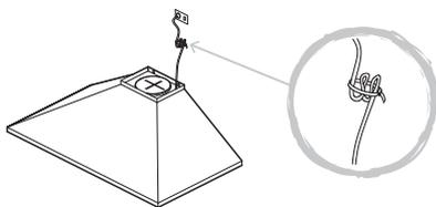
Once the electrical connection point and routing of the mains cable is established ensure that any excess cable is secured in such a way to prevent it falling into the motor housing and damaging the appliance.
