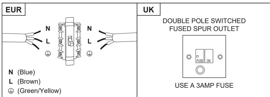
**The fuse must be rated at 3 Amps.**
