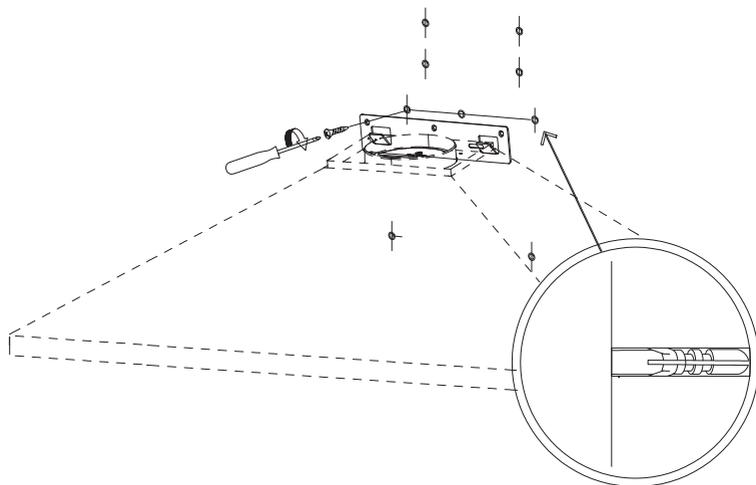
**EN** Install the hanging bracket on the wall with 3pcs flat head screws.
